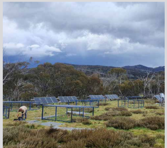
FutureClim: Climate control chambers for realistic, replicated, factorial field simulation of future warming & precipitation regimes.
